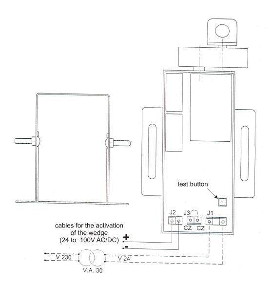
**TERMINAL BLOCK J2:** Connection for the wedge (From 24 to 100V DC/AC). Pay attention to the polarity of the connection
